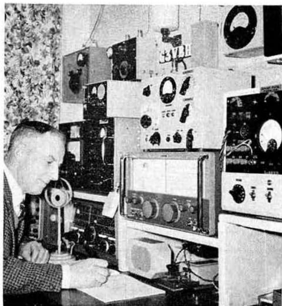
G3VBH, Bath, uses this fine array of equipment on all bands 10 to 160m. The transmitter above the Eddystone receiver is the one described in the Amateur Radio Handbook using a TT11 in the final stage
